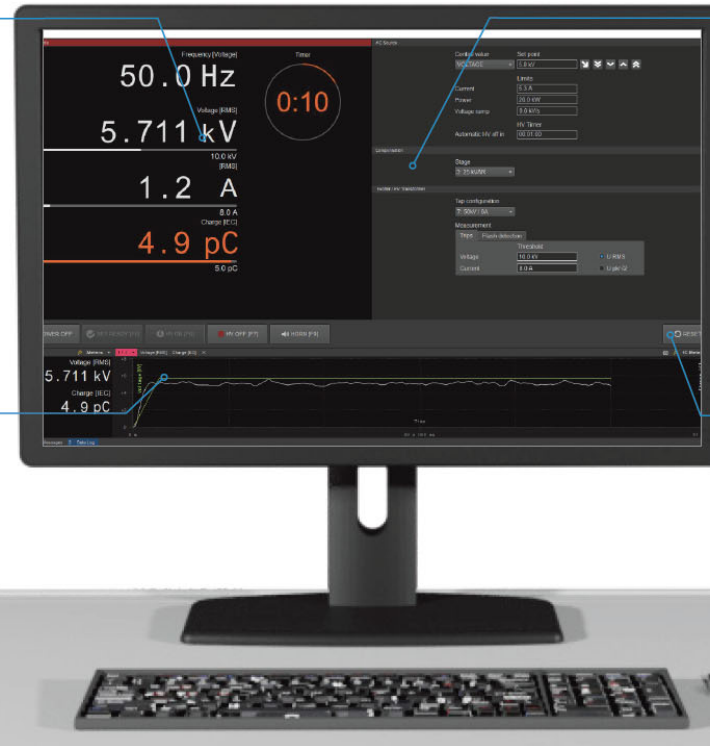
✓ Large Indicators Large numerical indicators with unit and bottom running range indication bar
