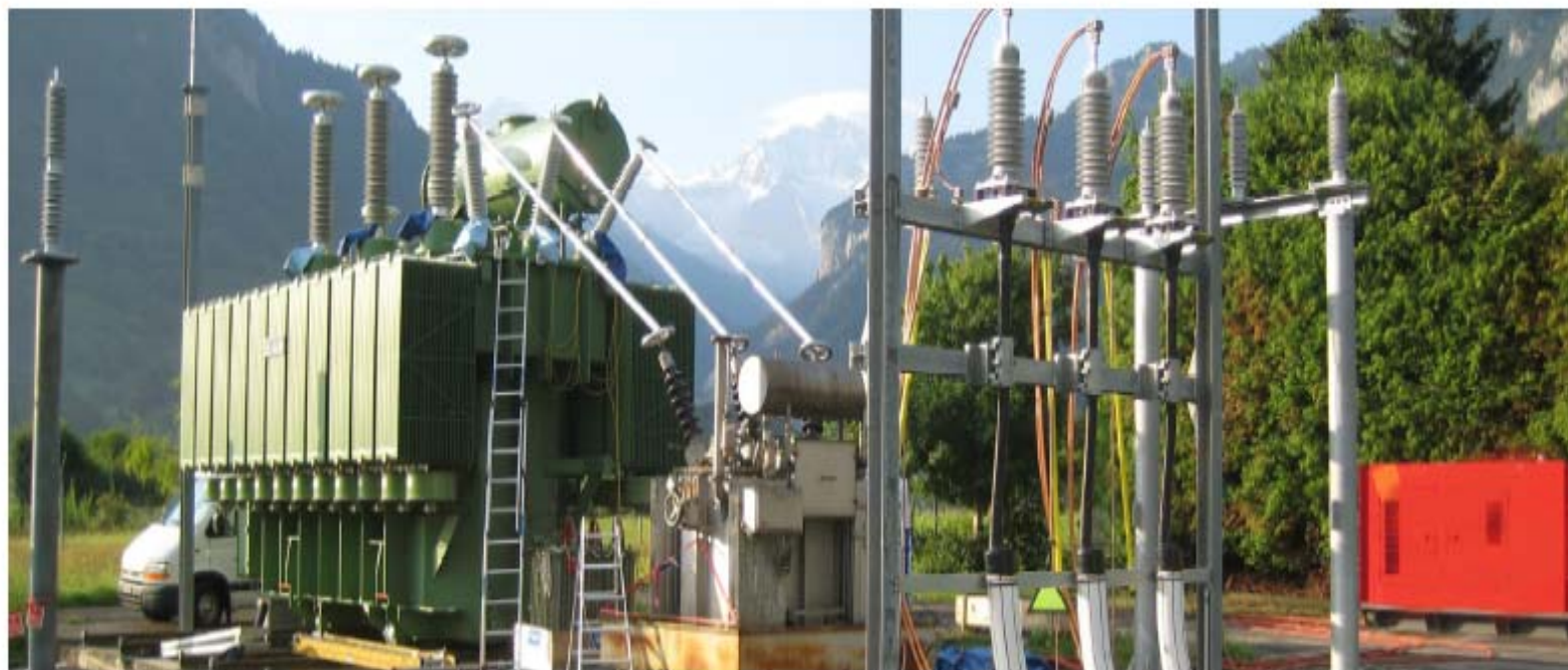
Figure 1: Example of an on-site test of a 75 MVA transformer (132/50 kV). In the middle the exit transformer (0.4/50 kV); on the right side (red box) the diesel generator (360 kVA).
