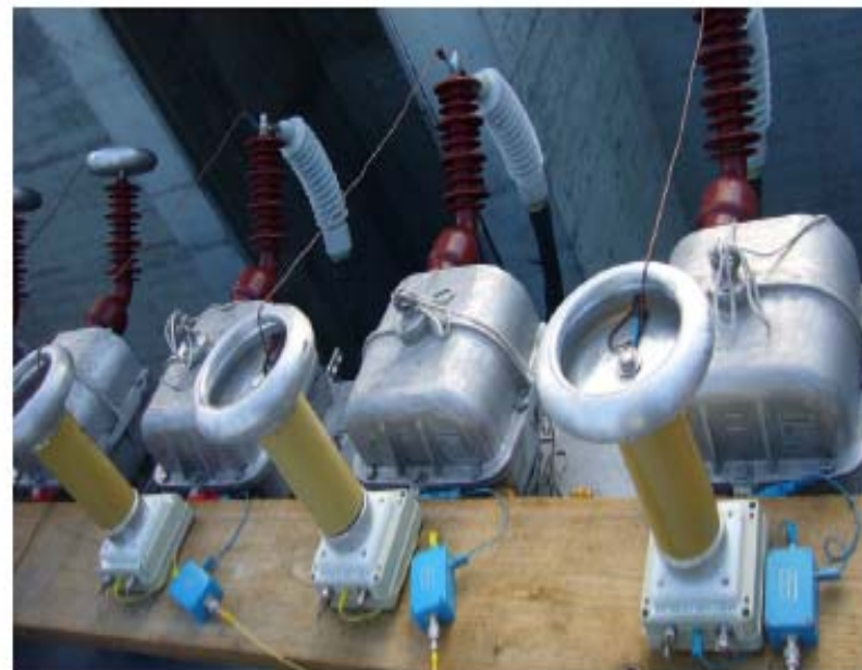
Figure 2: Connection of a high frequency current transformer (with secondary capacitance for voltage measurement) to the tap-off connector of a capacitor bushing (left); or use of external coupling capacitors (right)
