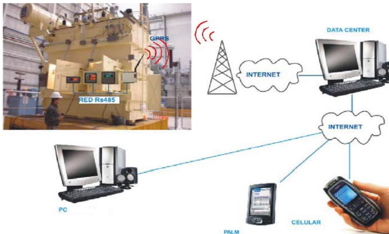
Figure 2. Schematic presentation of the wireless monitoring system. The sensors installed on the monitored transformer are of IED ( Intelligent Electronic Device ) type, and are directly connected to the short communication bus RS 485. Then, GSM ( Global System for Mobile Communication ) mobile-telephone transmitter sends them to the remote IDC ( Internet Data Center ) using GPRS ( General Packet Radio Service System ) protocol.
