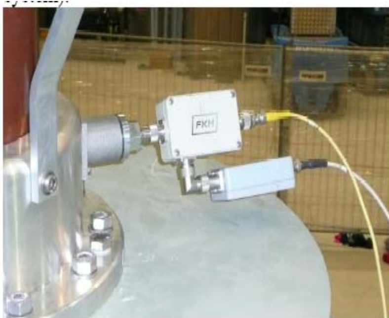
Figure 2: Connection of a high frequency current transformer (with secondary capacitance for voltage measurement) to the tap-off connector of a capacitor bushing (left); or use of external coupling capacitors (right)
