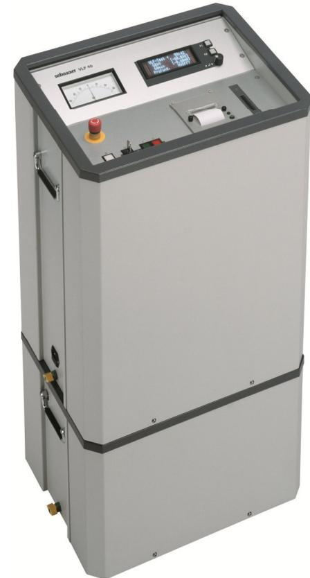
\* The leakage current indication gives the user a first indication about the quality of the insulation
