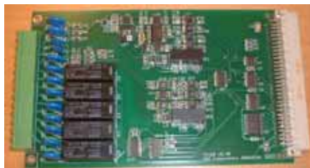
TC 160 Control and output 3 DO, Warning, Alarm & Trip
