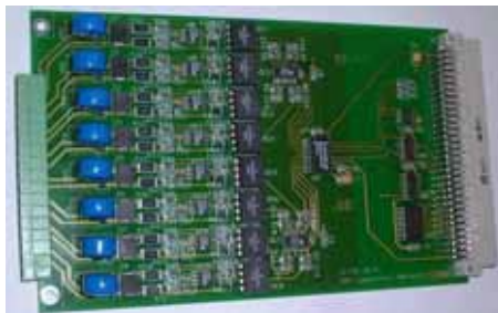
TC130, analogue 4-20 mA board (8 inputs)
