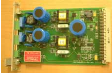
TC 110, power supply board Input 85-264 V AC and/or DC
